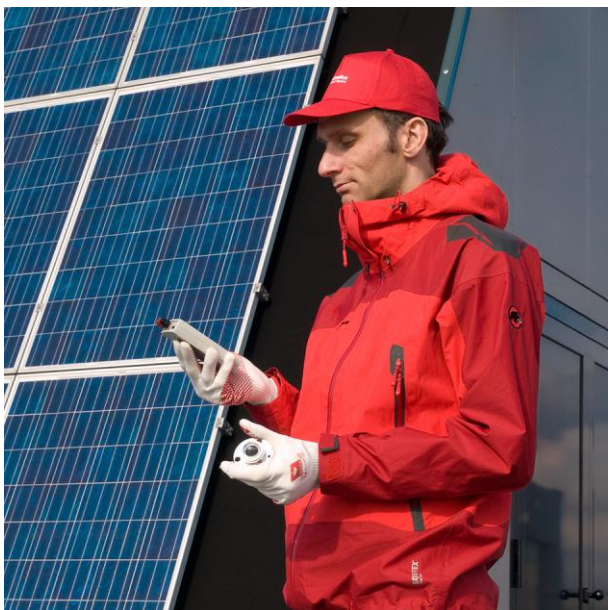
Figure 2 pyranometer in use with LI19 read-out unit
