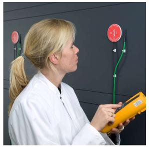
Figure 2 HFP01 heat flux sensor and TC mounted on a wall
