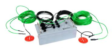
**Figure 1** *TRSYS01:* the complete measuring system includes 2 HFP01 heat flux sensors and 2 matched TC thermocouple pairs (in total 4 temperature sensors) and the MCU01 measurement and control unit
