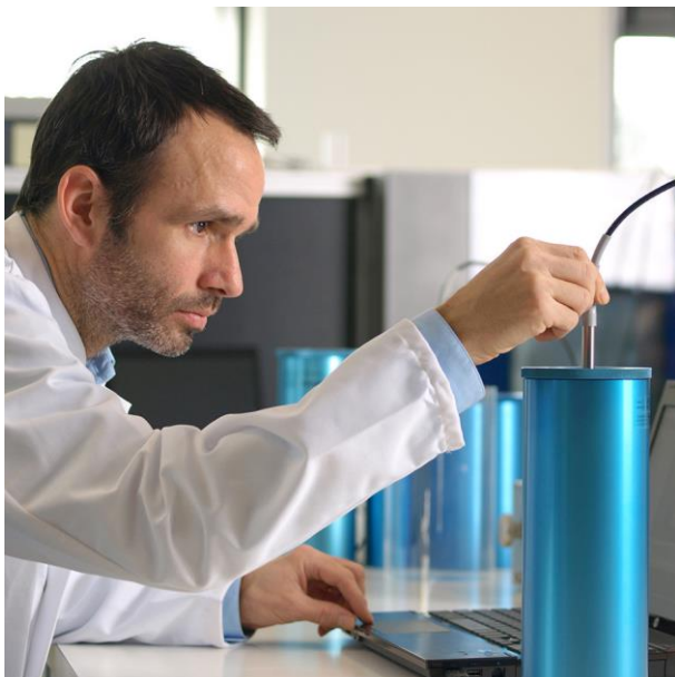
Figure 5 A calibration reference cylinder type CRC05 for needle calibration. The CRC05 is not included in the standard TNS02. For TNS02 two cylinders are required: CRC04 and CRC05.
