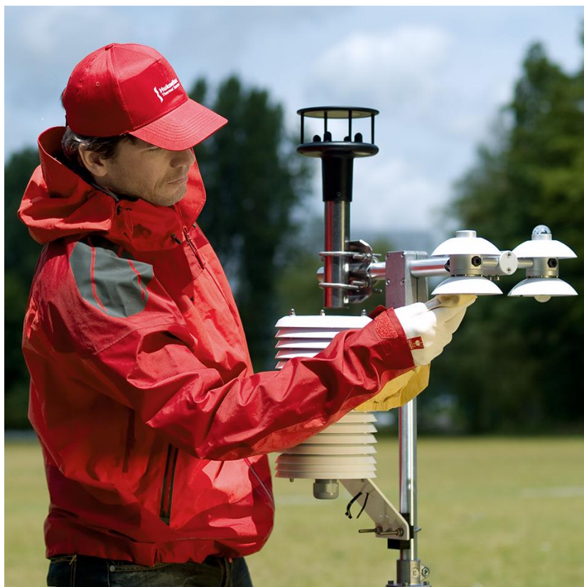
Figure 4.1 typical meteorological surface energy balance measurement system with STP01 installed in the soil
