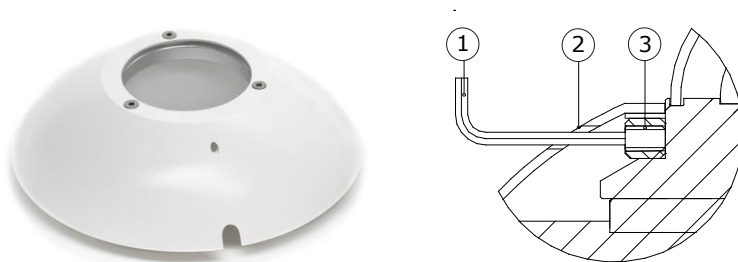
Figure 5.2.1 SCR01 sun screen and its installation and removal: turn the set screw using the hex key and lift off the sun screen to remove. (1) hex key, (2) sun screen, (3) set screw
