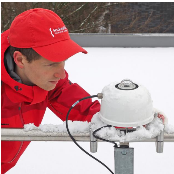
Figure 2 SR22 sensor combined with VU01 ventilation unit
