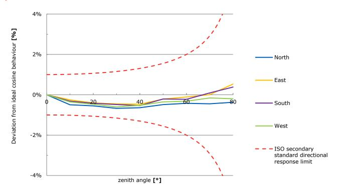
Figure 3 Directional response of a SR20 pyranometer of 4 azimuth angles, compared to secondary standard limits
