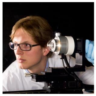
Figure 2 Directional response testing at Hukseflux
