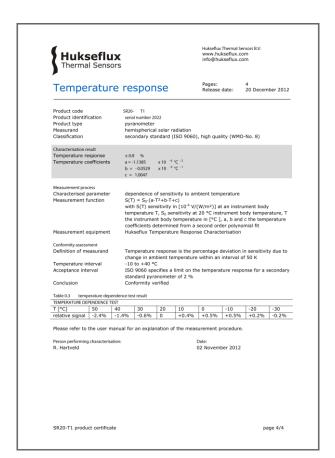
**Figure 3** The right paperwork. Test certificate of temperature response supplied with every individual instrument
