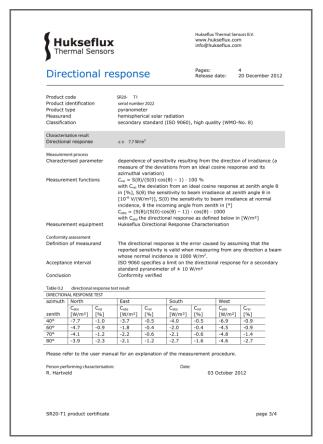
**Figure 5** The right paperwork. Test certificate of directional response supplied with every individual instrument
