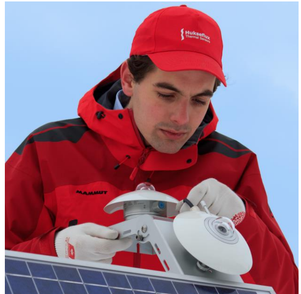
Figure 4 SR20-D2 secondary standard pyranometers with digital output for GHI (global horizontal irradiance) and POA (plane of array) measurements
