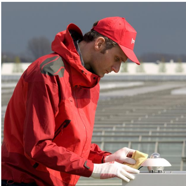
Figure 2 application example: solar sensor in use for greenhouse climate control; pyrgeometers are used for this application as well.
