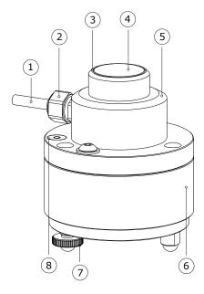
Figure 2 overview of IR02-TR: (1) cable, (2) cable gland, (3) window with solar blind filter, (4) sensor (below window), (5) sensor body, (6) transmitter housing (7) levelling feet, (8) bubble level
