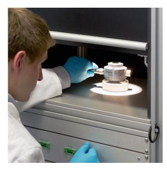
Figure 4 pyrgeometer during conformity assessment
