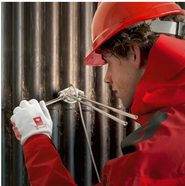
Figure 2 Example of an industrial heat flux sensor mounted on a boiler wall using tack-welded threads and spring-loaded bolts. The sensor is mounted on a well-prepared flat surface. Cabling must be provided with strain relief.
