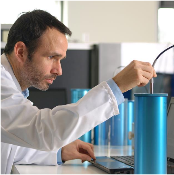
Figure 6 Laboratory measurements with thermal needle model TP02 and CRC Calibration Reference Cylinders
